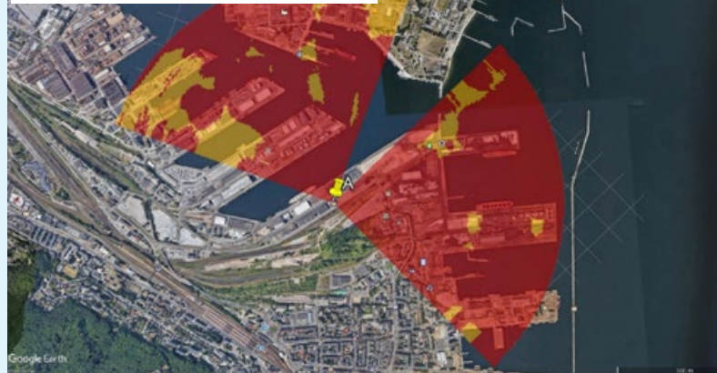
Recommended radar configuration Height above the radar - 50m Drone - DJI Matrice 600
