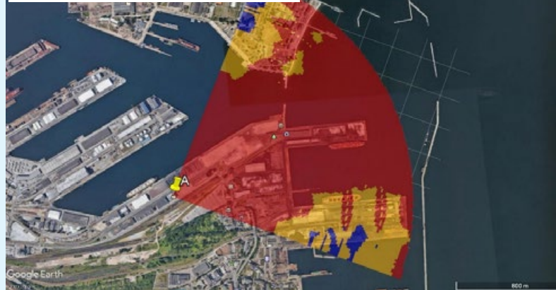
Radar coverage prediction map - Azimuth 65° Height above the radar - 50m Drone - DJI Matrice 600
